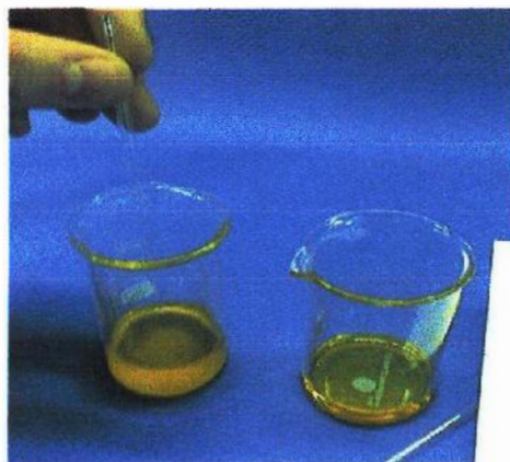
Fig.5 Capillary tube as sample spotter
