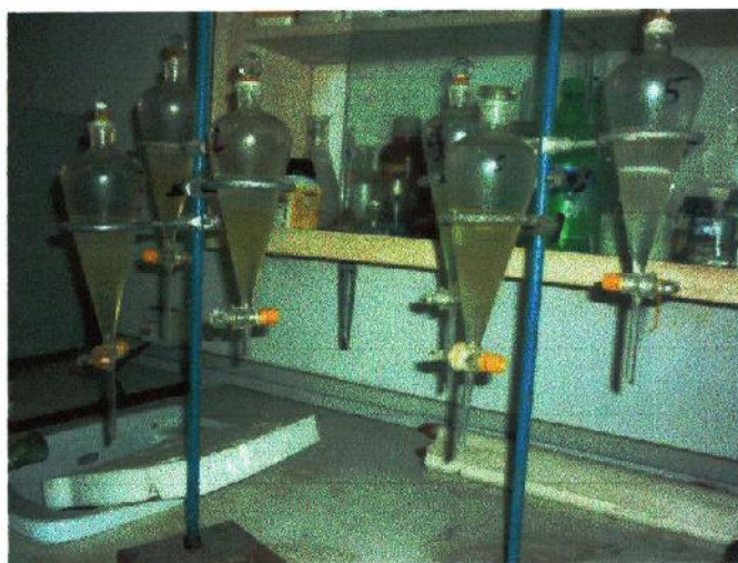
3: Lipid separation funnel
