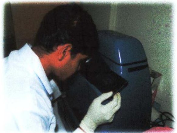
Figure: Observing bands under UV transilluminator
