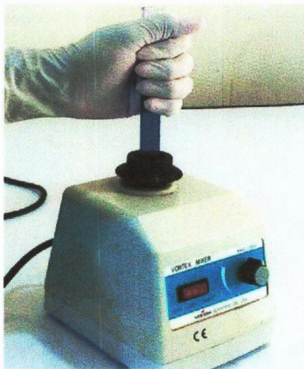
Figure 6. Mixing of sample with culture media in Vortex mixer
