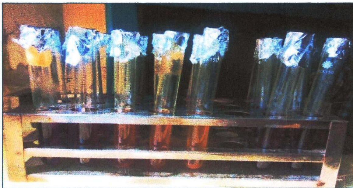
Figure 2.4 Estimation of the number of positive tubes out of all the tubes for each of the dilution separately
