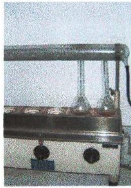
Plate 6: Two apparatus of Kjeldal method of protein determination from the muscle of A. testudineus
