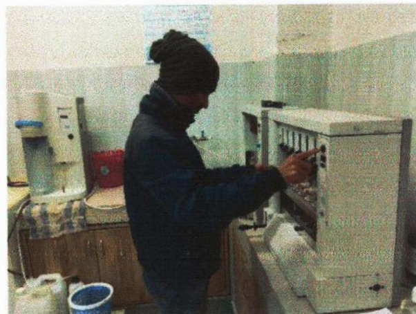
Figure 7.25 Ongoing ether extract test
