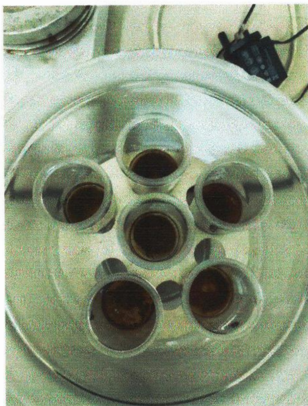
Figure 7.26 Vessels with sample inside desiccator for complete moisture removal for ether extract test
