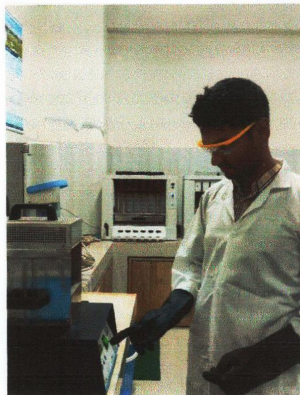
Figure 7.27 Ongoing digestion process for crude protein determination
